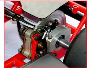
Handy Split bearing housings and twin cable operated disc brake
