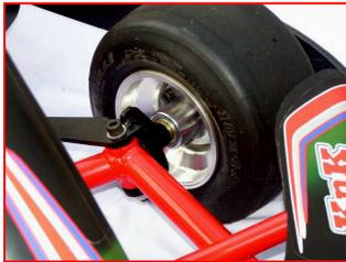
Heavy duty Knuckle with 20mm Stub Axles - replaceable.
